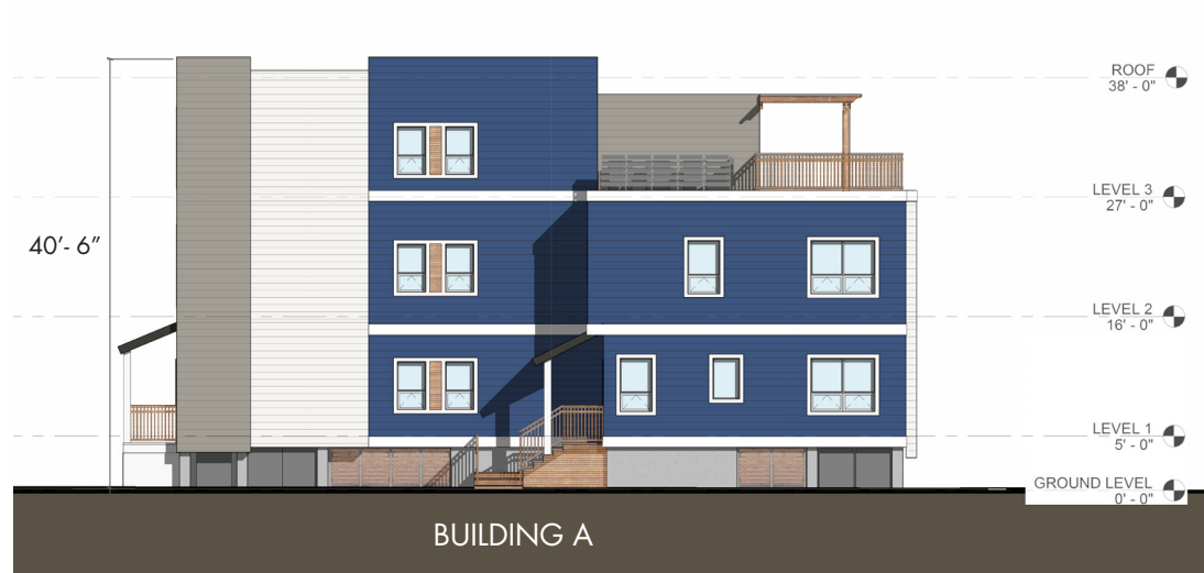
BUILDING A | EAST ELEVATION - VIEW 5
